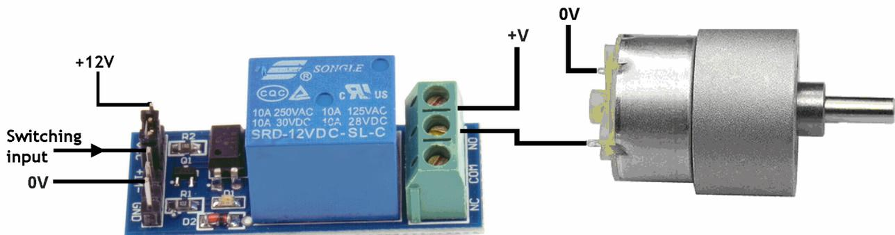
The top pin (labelled as VCC) is connected to +12V and the bottom pin (labelled as GND) is connected to 0V. The third pin from the bottom is the input to the module and it connects to whatever you are using to switch the circuit.
