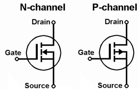
Unlike bipolar transistors, MOSFETs are voltage controlled. The field-effect transistor is a type of transistor that uses an electric field to control the flow of current. Whereas the bipolar transistors use a base-emitter current to control output current, the FET has almost no gate-source current flow.
