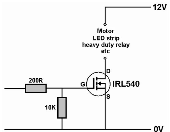
The 200 Ohm resistor is there to protect the attached circuit should the MOSFET fail and to limit any instantaneous high current when the transistor is first switched on (the gate can be highly capacitive and produce a brief current surge). The 10k Ohm resistor ensures the gate turns off when Gate signal is removed.
