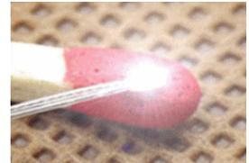
They use very thin flexible Micro Litz leads, allowing easy installation in vehicles, signals, traffic lights, etc.
