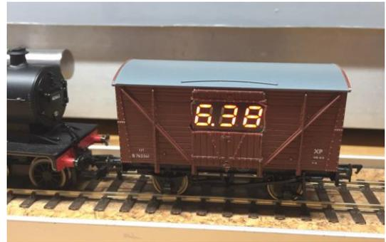
Showing DCC system voltage (*Lenz system*)
