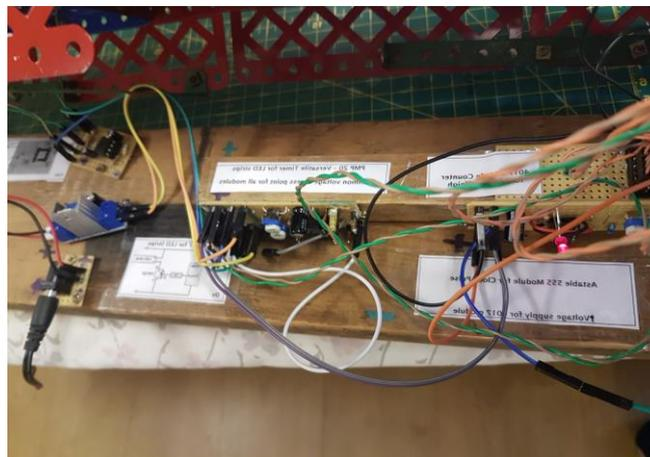
The power is via [LM317 DC-DC Converter Buck Step Down Module Linear Regulator Adjustable Voltage Regulator Power Supply Board](#) 5 for £3.31 seemed to me a pretty reasonable price! Rated at 1.5A there should be no problems with current usage for combining these applications to run from this one power source.
