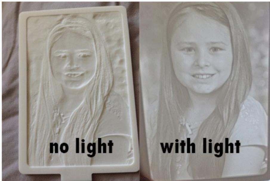
**Figure 2** : Typical 3D printed flat Lithophane
