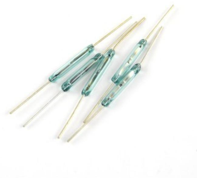
You can buy latching reed relay switches at considerable expense, or you can use a simple cheap reed relay element and set a bias magnet a few mm away to turn it into a latching relay.
