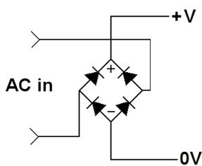
Some loco controllers have an auxiliary 15V or 16V AC output and the **PMP6** kit takes this output and converts it to a more beefy 12V 1A DC supply.
