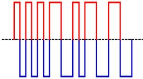
A DCC signal is bi-polar, constantly changing polarity and placing two diodes in the DCC path allows the DCC signal to always pass through regardless of the polarity
