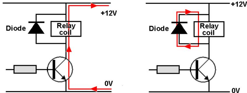
When the transistor is switched off, the magnetic field round the relay coil collapses and induces a high voltage in the opposite direction. Without the diode this reverse voltage could damage the rest of the circuit. The illustration on the right shows the effect of adding the diode; it provides a safe discharge path.
